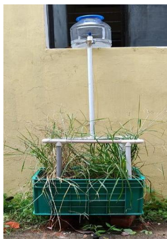
Figure 6: Constructed wetland unit
